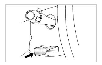
To tilt the wheel, hold the wheel and pull the lever. Then move the wheel to a comfortable position and release the lever to lock the wheel in place.
